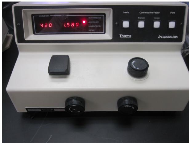
Figure 7. A spec 20 used to determine cell density. Here the spectrophotometer is set to a wavelength of 420 nanometers (nm).
