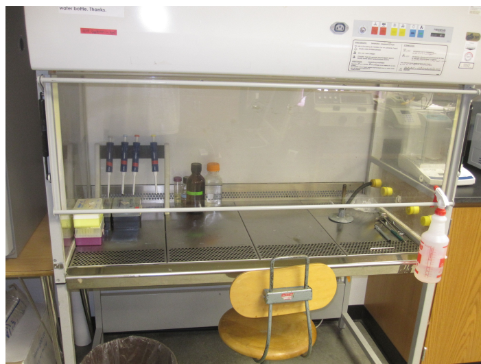
Figure 1. A laminar flow hood where media is prepared or cultures can be manipulated in sterile conditions.
