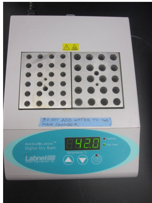
Figure 10. A heat block is often used to regulate reactions in microcentrifuge tubes such as cutting DNA. Here the heat block has been set to 42.0°C.
