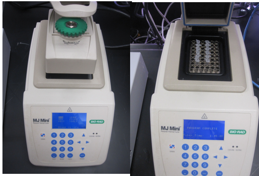
Figure 6. A thermocycler with its lid almost closed and ready to start (left). After the PCR has completed the lid is opened (right) and the PCR tubes are removed.
