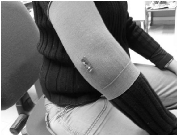
FIGURE 3.22 Application of a field-effect strain sensor to the elbow joint bending detection.
