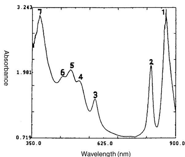
**Figure 1.** Absorption spectrum of whole cell suspensions of isolated strain B1. Peak 1 = 863 nm; peak 2 = 806 nm; peak 3 = 591.5 nm; peak 4 = 529.5 nm; peak 5 = 498 nm; peak 6 = 470.5 nm; peak 7 = 378 nm.
