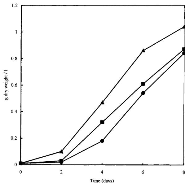
**Figure 3.** Effect of yeast extract supplementation on the growth of strain B1 in 50% effluent diluted in BM medium. 0% Yeast extract (●), 0.01% yeast extract (■) and 0.1% yeast extract (▲).
