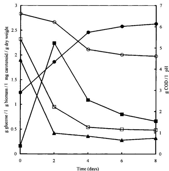
**Figure 4.** Growth profile and carotenoid contents of strain B1 in relation to certain physicochemical characteristics of the sago effluent medium, under anaerobic-light conditions. Biomass (●), pH (○), total carotenoid (■), chemical oxygen demand (□) and total carbohydrate (▲).
