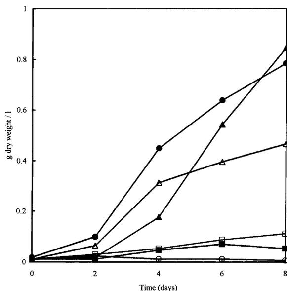
**Figure 2.** Effects of effluent concentration and mineral supplementation on growth of strain B1 in sago effluent medium. BM medium without carbon source (○), BM medium with carbon source (●), 25% effluent diluted in water (□), 50% effluent diluted in water (■), 25% effluent diluted in BM medium (△) and 50% effluent diluted in BM medium (▲).
