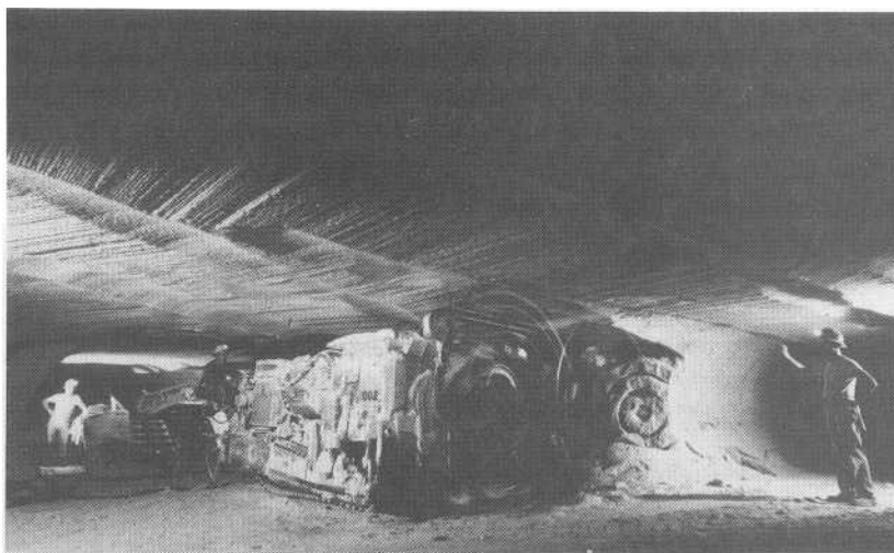
FIGURE 14.6 A continuous mining machine at work about 1 kilometer underground in potash mine at Esterhazy, Saskatchewan, Canada. (Photograph courtesy American Potash Institute and International Minerals and Chemical Corporation.)
