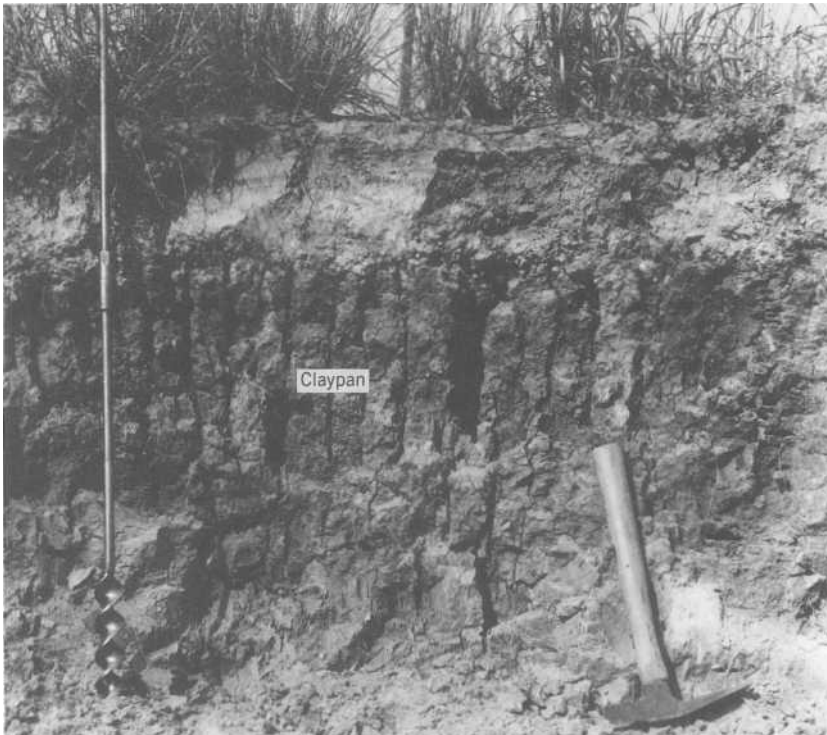
FIGURE 3.6 A soil with a strongly developed Bt horizon; a claypan. On drying, cracks form between structural units. On wetting, the soil expands, the cracks close, and the claypan becomes impermeable to water and roots. (Photograph courtesy Soil Conservation Service, USDA.)
