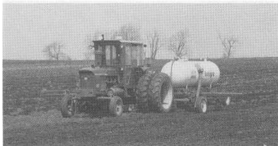
FIGURE 14.2 Injection of anhydrous ammonia into soil. The ammonia is handled as a liquid under pressure.
