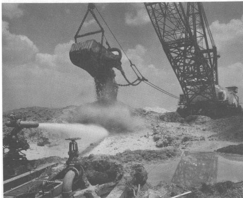
FIGURE 14.4 Mining rock phosphate. The overburden is removed and a hydraulic gun is used to break up the ore layer and form a slurry that is pumped to a recovery plant. (Photograph courtesy International Minerals and Chemical Corporation.)
