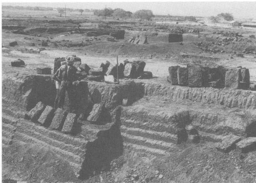
FIGURE 18.21 Mining plinthite in Orissa state, India. On drying, the bricks harden and are used for construction.
